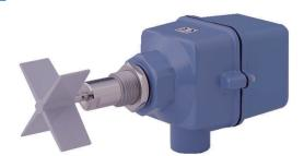
R7 is a solid level measurement sensor that is ideal to incorporate in plastic processing machinery or cereal processing machinery. The sensor has a paddle that is projected to the tank and rotates slowly. Without material around the paddle, it keeps rotating. When material reaches the paddle, the rotation stops and the output signal is given.
