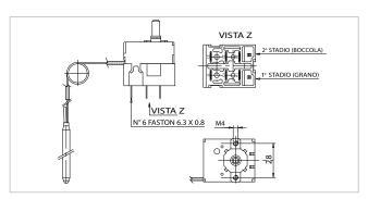
Electrical contact capacity = 15 (2,5) A / 250 Vac Switches = changeover Max. head temperature = 80°C Capillary length = 1500 mm PVC Min. capillary curvature radius = 5 mm Connection = via faston Certifications = CE, ENEC03, EAC
