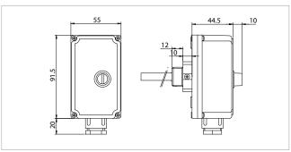
Electrical contact capacity = 10(2,5) A / 250 Vac Switches = interrupted due to temperature increase Thermal gradient = 1°K/min Max. head temperature = 80°C Max. bulb temperature = 125°C Protection rating = IP40 Certifications = CE, ENEC03, DIN, PED, EAC
