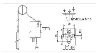
Electrical contact capacity = NC 16(6) / A 250 Vac Switches = changeover Max. head temperature = 85°C Min. capillary curvature radius = 5 mm Connection = via faston 6,3x0,8 Certifications = CE, ENEC03, EAC, UL, CSA
