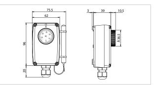
Differential = from 3 to 6°C Electrical contact capacity = 16(2,5) A / 250 Vac Max. operating temperature = 65°C Protection rating = IP54 Certifications = CE, ENEC03, EAC
