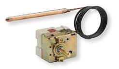
TRZ is a capillary thermostat with liquid expansion probe and 2-stage switch, unipolar, with switching contacts, particularly suitable for automatic temperature regulation for applications in civil and industrial heating, air conditioning and household appliances such as radiators electric, boilers, washing machines, dishwashers, etc.
