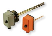
LSC1 is a boxed immersion thermostat, with liquid expansion probe, unipolar, safety temperature limiter with manual reset, failsafe for capillary breakage, complete with watertight protection pocket. Useful in appliances where safety is required due to the temperature increase.
