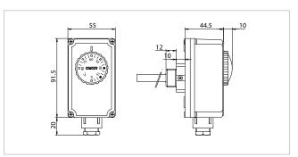
Electrical contact capacity = 10(2,5) A / 250 VacSwitches = interrupted due to temperature increase or exchange Max. head temperature =  $80^{\circ}\text{C}$ Max. bulb temperature =  $125^{\circ}\text{C}$ Thermal gradient =  $1^{\circ}\text{K/min}$ Protection rating = IP40 Certifications = CE, ENECO3, DIN, PED, EAC
