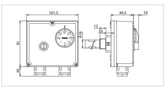
Electrical contact capacity = 10 (2,5) A / 250 Vac Switches = interrupted due to temperature increase or exchange Max. head temperature =  $80^{\circ}$ C Max. bulb temperature =  $125^{\circ}$ C Thermal gradient =  $1^{\circ}$ K/min Protection rating = IP40 Certifications = CE, ENECO3, DIN, PED, EAC
