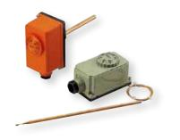
TC2 is a boxed immersion thermostat with liquid expansion, unipolar, with changeover switches, complete with a watertight protection pocket. The thermostat normally applied on delivery piping is particularly suitable for the automatic regulation of boilers, pumps and other various appliances. It is also available in a capillary version.
