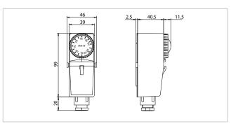
Differential =  $8\pm 3K$ Electrical contact capacity = 16(2,5) A / 250 VacThermal gradient =  $1^{\circ}K/\text{min}$ . Max. head temperature =  $80^{\circ}C$ Protection rating = IP20 Certifications = CE, ENEC03, EAC
