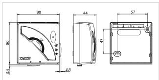
Power supply = 230 Vac Regulation range = 7°÷30°C Differential = 1 K Thermostat contact capacity = 16(2,5) A / 250 Vac Selector switch capacity = 10(2) A / 250 Vac Output = changeover switches Installation = wall Operating mode: Summer/Winter/Anti-freeze System: fan-coil/radiators/fan convectors Certifications = CE, ENEC03, EAC
