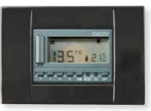
FAN 503 is an electronic built-in DIN503 regulator for fan coils, radiators and fan convectors with LCD display. It includes three relays to regulate the fan speed and two relays to control the solenoid valves and the water probe inlet (NTC 10K probe included in the package).
