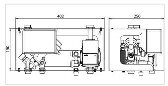
Supply voltage = 230 V / 50 HzMax. absorbed power = 50 WOperating water temperature =  $0/95^{\circ}\text{C}$ Working room temperature =  $0/60^{\circ}\text{C}$ Storage temperature =  $0/60^{\circ}\text{C}$ Max. heating fluid pressure = 3 barMax. fluid pressure ACS = 6 barProtection rating = IPX4D Certifications = CE
